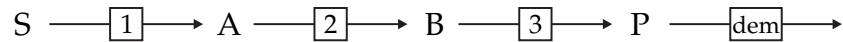
Figure 42: A linear metabolic supply-demand system. The biosynthetic supply consists of three steps, which convert the substrate S to the product P via the intermediates A and B. The demand is a single reaction consuming P.
